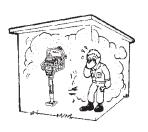
enclosed or narrow area where free flow of the air is restricted. If the air flow is restricted it will cause serious damage to the rammer or engine and may cause injury to people. Remember the rammer's engine gives off **DEADLY** carbon monoxide gas.
